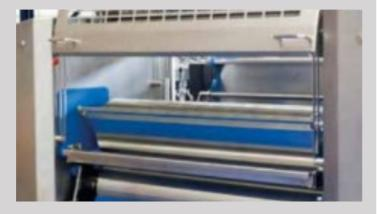
are applied which can be lubricated during or after the production run. To keep the rollers of the reduction stations as clean as possible they are fitted with wear resistant roller scrapers which were selected after extensive testing.
