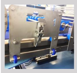
Convenient rollers on the tooling modules enables change-over without the risk for damaging the conveyor belt. Lightweight safety covers with extra handles enable ergonomic operation.
